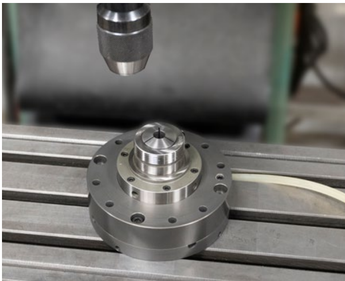
Dunham Air Collet Chuck in Stationary Mount for Milling Operation
