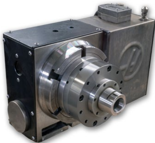
Air Chuck Mounted on 4th Axis Indexer
